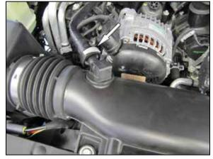
3. Disconnect the crank case vent line.
