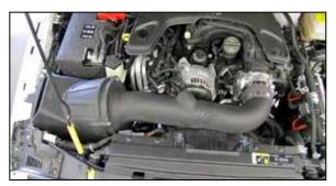
17. Install the K&N® intake assembly into the hose at throttle body first, then engage the K&N® airbox mounts into the factory airbox mounting location. Secure K&N® intake assembly with provided clamp.
