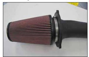
14. Install the K&N<sup>®</sup> air filter onto the K&N<sup>®</sup> intake tube.
