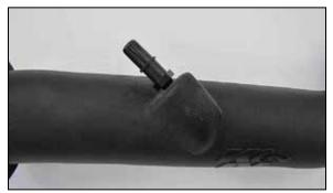
12. Install ¼ NPT quick connect fitting onto the tube.
