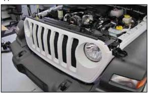
10. Reinstall the grill reengaging the lower clips one at a time then reinstall the six clips that hold the grill to the top of the core support.
