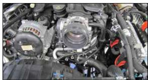
16. Install provided hose onto the throttle body (08171) secure with provided clamp.
