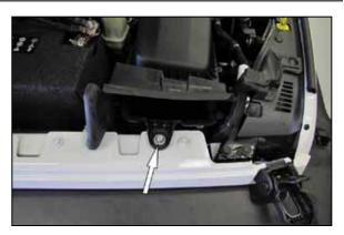
5. Remove the bolt that secures the factory air box to the fender and remove assembly from the vehicle.
