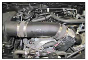
9. Lift up the upper air filter housing, install the K&N® intake tube into the coupling hoses and then reinstall the air filter housing. Secure the air filter housing with the factory clips, adjust the intake tube for best fit and then secure with the provided hose clamps.
