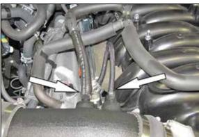
11. Connect the union into the factory crank case vent hose and then connect the open end onto the fitting installed into the K&N® intake tube. Then connect the fuel pressure regulator vent hose to the fitting installed in the K&N® intake tube.
