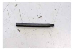
10. Install the provided hose union into the provided crank case vent hose.
