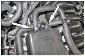
3. Disconnect the crank case vent hose and fuel pressure regulator vent hose from the factory intake tube.
