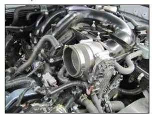
8. Install the provided coupler hose (08690) onto the throttle body and secure with the provided hose clamp.
