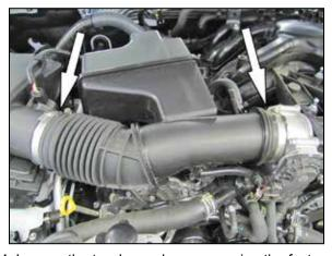
4. Loosen the two hose clamps securing the factory intake tube and then remove the intake tube from the vehicle.
