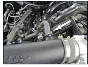
11. Connect the factory crank case vent hose to the fitting installed into the K&N<sup>®</sup> intake tube and secure with the factory spring clamp.
