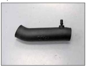
9. Install the provided NPT vent fitting into the  $K\&N^{\scriptsize @}$  intake tube as shown.
