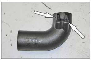
9. Install the provided vent fittings into the K&N<sup>®</sup> intake tube as shown.
