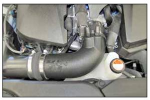
10. Install the K&N<sup>®</sup> intake tube assembly into the coupler at the air filter housing and then into the coupler at the throttle body. Adjust the tube for best fit and then secure with the provided hose clamps.
