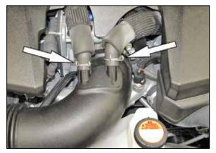
2. Release the spring clamps securing the crank case breather hoses and then disconnect the hoses from the intake tube.
