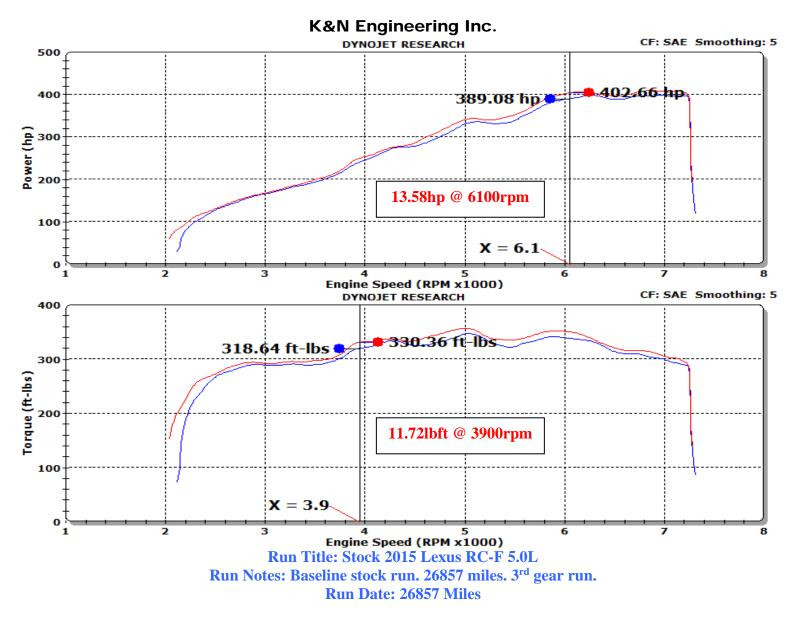
Run Title: K&N 2015 Lexus RC-F 5.0L Run Notes: K&N intake kit #63-9038 installed. 26857 miles. 3<sup>rd</sup> gear run. Run Date: 9/28/2016 9:09:47 AM K&N.002: 90.69 °F 28.97 in-Hg Humidity: 23 % SAE: 1.04
