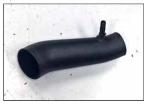
8. Install the provided combination vent fitting into the K&N® intake tube as shown.
