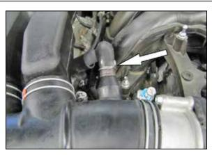
3. Release the spring clamp and then disconnect the crank case vent hose from the factory intake tube.
