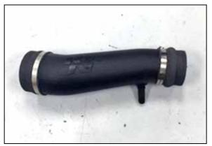
9. Install the provided coupler hoses onto the K&N<sup>®</sup> intake tube as shown and secure with the provided hose clamps.
