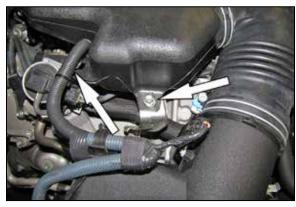
4. Remove the bolt which secures the intake plenum to the mounting bracket and unhook the mass air sensor wiring harness from the intake plenum.
