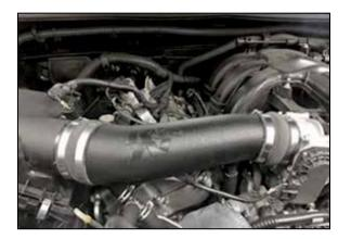
12. Adjust the intake tube for best fit and then secure with the provide hose clamps.
