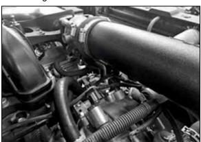
14. Connect the crank case vent hose to the fitting installed into the K&N® intake tube and secure with the factory spring clamp. Install the supplied fuel pressure regulator vent hose into the factory vent hose and then connect it to the small port of the fitting installed into the K&N® intake tube.
