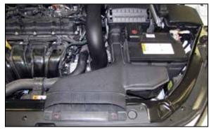
17. Reinstall the fresh air intake duct and secure with the factory bolts.
