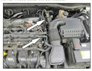
4. Disconnect the EVAP vent hose from intake tube and then disconnect the crank case vent hose from the valve cover.
