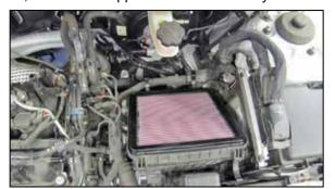
8. Install the provided K&N® air filter and then reinstall the upper air box and latch into position.
