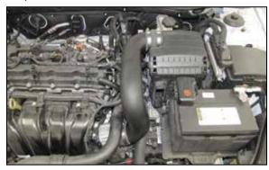
15. Install the intake tube assembly into the coupling hose at the throttle body and then into the hose at the air box, secure the tube with the provided hose clamps.
