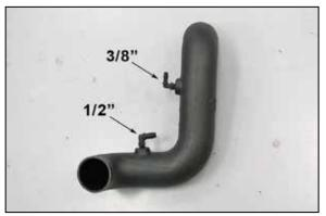
9. Install the two provided 3/8" and  $\frac{1}{2}$ " 90\* vent fittings into the K&N® intake tube as shown. NOTE: Plastic NPT fittings are easy to cross thread. Install the vent fitting "hand" tight, then turn it two complete turns with a wrench.
