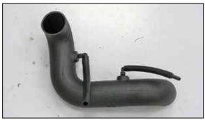
12. Install the provided  $\frac{1}{2}$ " vent hose onto the  $\frac{1}{2}$ " fitting as shown.
