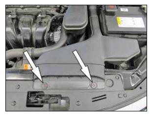
3. Remove the two bolts securing the fresh air intake duct to the core support and then remove the fresh air intake duct from the vehicle.
