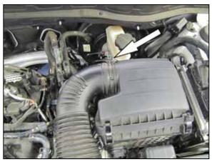
6. Loosen the hose clamp securing the factory intake tube to the air box and then remove the intake tube from the vehicle.
