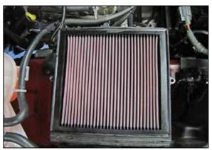
6. Replace the factory air filter with the K&N® air filter provided. Reinstall the upper air filter housing and secure with the factory screws.
