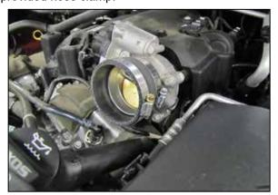
8. Install the provided coupler (08186) onto the throttle body and secure with the provided hose clamp.
