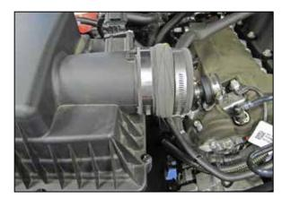
7. Install the provided hump coupler (08171) onto air filter housing outlet and secure with the provided hose clamp.
