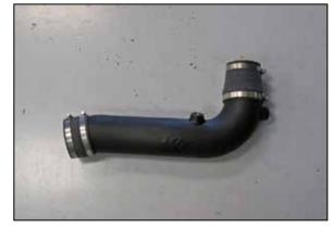
6. Install the provided coupler hoses onto the K&N® intake tube and secure with the provided hose clamps.
