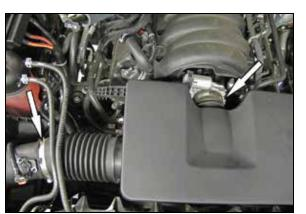
3. Loosen the hose clamps that secure the intake plenum to the throttle body and air filter housing. Then remove the intake plenum from the vehicle. NOTE: K&N Engineering, Inc., recommends that customers do not discard factory air intake.
