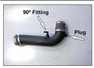
7. Install the provided 90° vent fitting and 1/4npt plug into the K&N® intake tube as shown.
