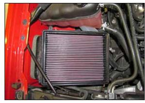
5. Install the K&N® air filter into the lower filter housing and then reinstall the upper housing and secure with the factory hardware.
