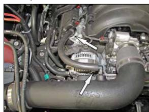
10. Install the crank case vent hose assembly onto the vent fitting installed into the K&N® intake tube and then connect the quick connect fitting to the port on the valve cover.
