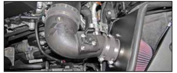
18. Install the K&N® intake tube into the hose at the filter adapter and then into the hose at the turbo chamber, adjust the tube for best fit and then secure with the provided hose clamps.
