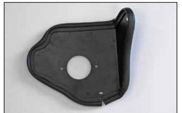
5. Install the provided edge trim onto the heat shield as shown.
