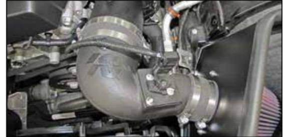
19. Reconnect the mass air sensor electrical connection and secure the wiring harness to the insert in the K&N® intake tube.
