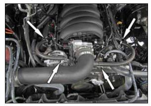
10. Install the crank case vent hose assemblies onto the vent fittings installed into the K&N<sup>®</sup> intake tube and then connect the quick connect fittings to the port on the valve covers.
