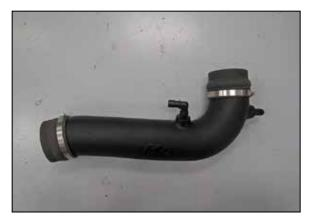
7. Install the provided coupler hoses onto the K&N<sup>®</sup> intake tube and secure with the provided hose clamps.
