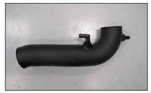
6. Install the provided 90° and straight vent fittings into the K&N<sup>®</sup> intake tube as shown. NOTE: Plastic NPT fittings are easy to cross thread. Install the vent fitting "hand" tight, then turn it two complete turns with a wrench.
