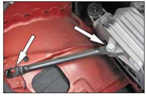
8. Remove the engine mount brace bolt and loosen the nut shown.
