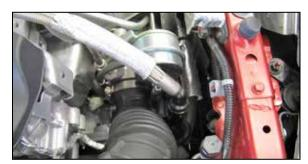
3. Disconnect the crank case vent hose.
