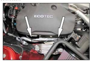
20. Using the provided tie wraps, secure the mass air sensor electrical cable to the A/C line as shown.
