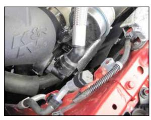
18. Connect the crank case vent hose to the fitting installed into the K&N<sup>®</sup> intake tube.
