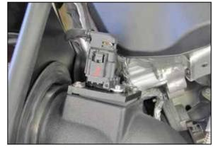
Reconnect the mass air sensor electrical connection.
