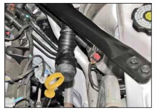
8. Install the caplug assembly into the remaining sound tube and secure with the provided tie wrap.
