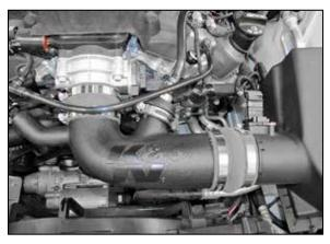
16. Connect the crank case fitting onto the K&N<sup>®</sup> intake tube and secure with the provided hose clamp.
