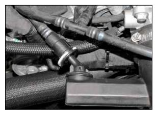
3. Release the locking tap and then disconnect the EVAP vent line quick disconnect fitting from the factory intake tube.
