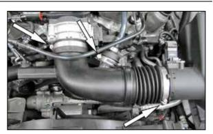
5. Loosen the three hose clamps that secure the intake tube and crank case vent tube and remove the intake tube from the vehicle.
