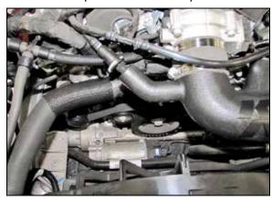
15. Connect the factory EVAP hose quick connector to the quick connector installed into the K&N® intake tube.
