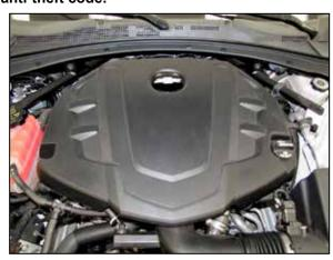
2. Remove the bolt that secures the decorative engine cover, remove the oil cap and then remove the decorative engine cover. Reinstall the oil cap.
