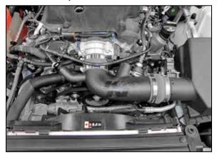
14. Install the K&N® intake tube into the coupling hose at the air box and then into the coupler at the throttle body, adjust the tube for best fit and then secure with the provided hose clamps.
