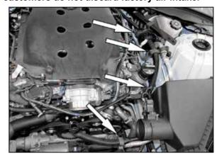
6. On vehicles equipped with an engine sound tube, release the three flexible clamps that secure the sound tube and disconnect the sound drum from the rear sound tube then remove the sound tube assembly. On vehicle that are not equipped with the engine sound tube, skip to step #9.
