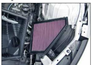
10. Remove the upper air filter housing and replace the factory air filter with the provided K&N® air filter. Reinstall the factory air filter housing and secure with the factory screws.
