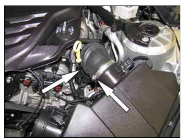
5. Loosen the hose clamps that secure the driver's side factory intake tube and then remove the tube from the vehicle.
