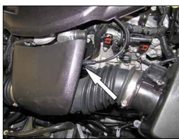
3. Release the crank case vent hose quick disconnect fitting and then disconnect the crank case vent from the factory intake tube.
