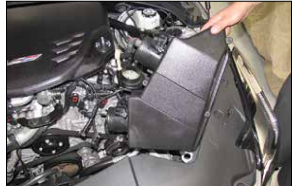
6. Lift the air filter housing assembly to dislodge it from the mounting grommets and then remove it from the vehicle.
