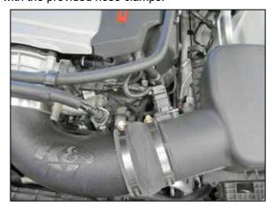
15. Connect the crank case vent hose to the quick connect fitting in the K&N® intake tube.
