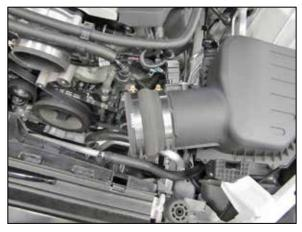
12. Install the provided hump coupler (08695) onto the mass air sensor and secure with the provided hose clamp.
