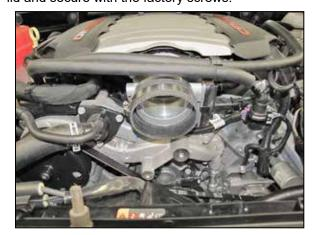
11. Install the provided coupling hose (08761) onto the throttle body and secure with the provided hose clamp.
