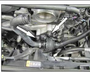
5. Remove the two bolts securing the sound drum to the engine.
