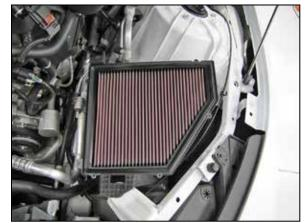
10. Install the provided K&N® air filter. Reinstall the lid and secure with the factory screws.
