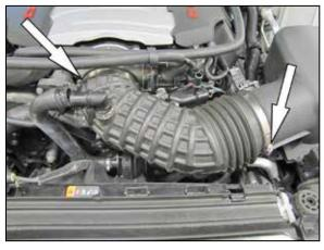
4. Loosen the two hose clamps and then remove the intake tube from the vehicle.
