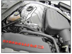
6. Disconnect the clamps securing the sound tube then disconnect the front sound tube from the rear tube and the union.
