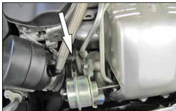
3. Loosen the hose clamp securing the intake tube to the turbo inlet.
