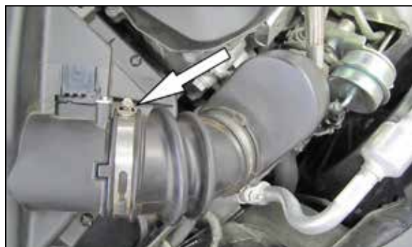
4. Loosen the hose clamp securing the intake tube to the air filter housing. Disconnect crankcase vent line from intake tube and remove tube from vehicle, then gently pull up air box assembly disengaging from grommets and remove from vehicle. NOTE: K&N Engineering, Inc., recommends that customers do not discard factory air intake.
