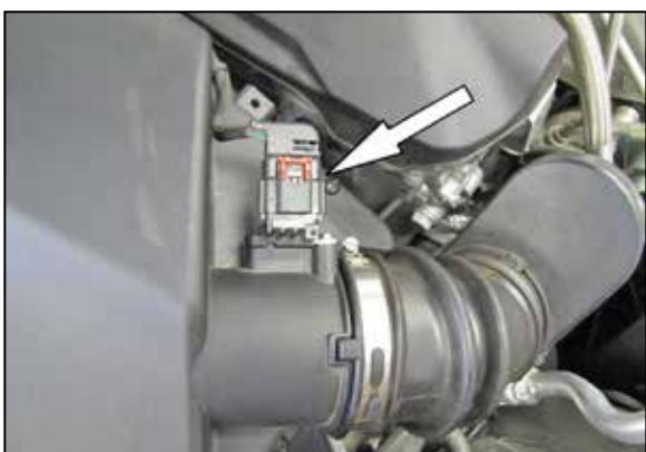
2. Disconnect mass air sensor electrical connector.
