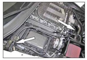
25. Install the provided crank case breather hose onto the fitting on the oil tank and then onto the fitting on the K&N<sup>®</sup> intake tube and secure with the provided spring clamps. Secure the hose as shown with the provided tie wraps.
