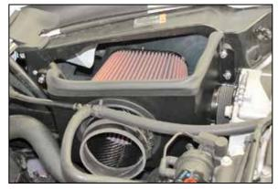
19. Install the heat shield/filter assembly onto the rubber mounted studs installed during step #15 and secure with the provided hardware.
