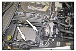
12. Install the previously assembled coolant hose assembly onto the expansion tank and then route it to the TEE fitting. Install hose onto the TEE fitting and secure with the provided spring clamp. Use the provided tie wraps to secure the hose where shown.
