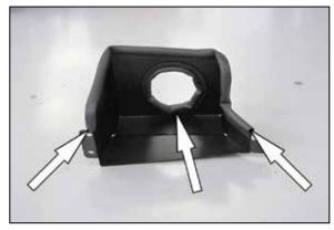
17. Install the 16" long edge trim into the hole of the heat shield and install the 27" long section around the edge of the heat shield as shown.
