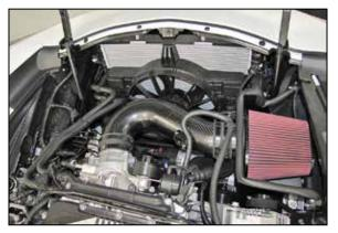
24. Install the K&N<sup>®</sup> intake tube into the heat shield and air filter and then into coupling hose at the throttle body. Adjust the tube and filter for best fit and then secure with the provided hose clamps.
