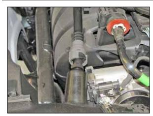
22. Connect the crank case vent hose to the fitting installed into the K&N® intake tube.
