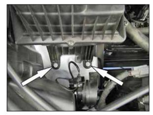
7. Remove the two nuts securing the air filter housing to the inner fender.
