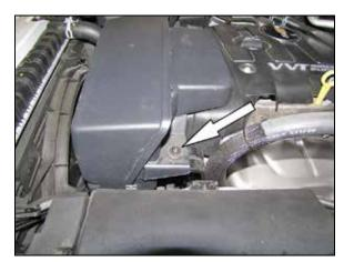
3. Remove the bolt that secures the intake plenum to the engine.
