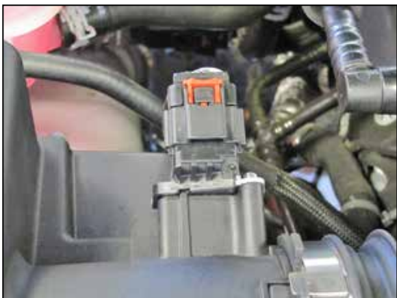
2. Disconnect the mass air sensor electrical connection.
