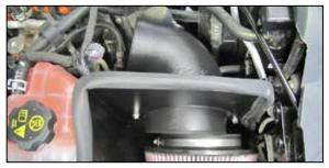
12. Install the K&N® intake tube into the heat shield and secure with the provided hardware and then install the K&N® air filter onto the K&N® intake tube and secure with the provided hose clamp.
