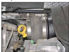
17. Install the provided hump hose (08633) onto the turbo inlet and secure with the provided hose clamp.
