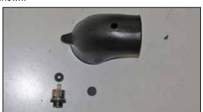
11. On vehicles equipped with a filter minder, remove the factory filter minder and grommet and install them into the K&N® intake tube. If the vehicle is not equipped with a filter minder install the provided plug into the K&N® intake tube.
