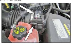
2. Disconnect the mass air sensor and humidity sensor electrical connections.
