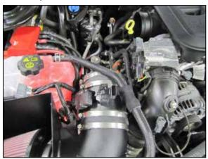
16. Install the Mass air assembly onto the K&N<sup>®</sup> intake tube as shown and secure with the provided hose clamps.
