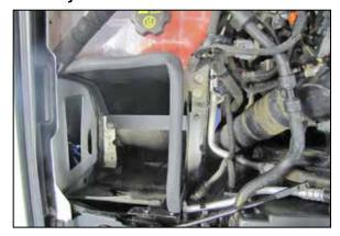
9. Install the K&N® heat shield onto the air box mounting plate and secure with three of the bolts removed in step #7.
