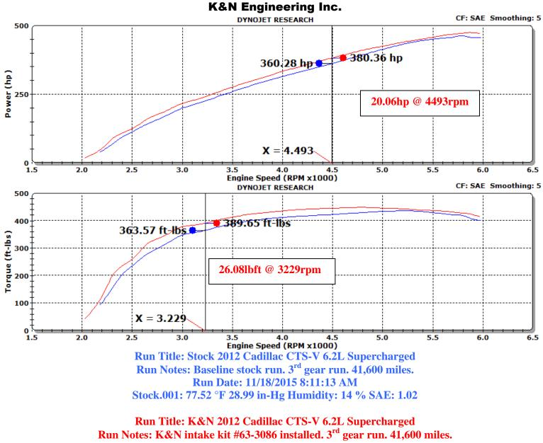
Run Notes: K&N intake kit #63-3086 installed. 3<sup>rd</sup> gear run. 41,600 miles Run Date: 11/18/2015 8:57:15 AM K&N.002: 81.17 °F 29.02 in-Hg Humidity: 13 % SAE: 1.02
