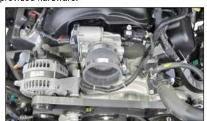
12. Install the provided step hose (084055) onto the throttle body and secure with the provided hose clamp.
