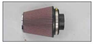
10. Install the filter adapter into the K&N<sup>®</sup> air filter and secure with the provided hose clamp.
