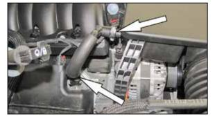
3. Disconnect the crank case vent from the intake plenum and valve cover port and remove it from the engine.
