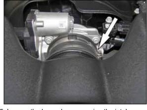
5. Loosen the hose clamp securing the intake plenum to the throttle body and then remove the intake plenum from the vehicle.
