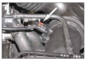
5. Disconnect the mass air sensor electrical connection.
