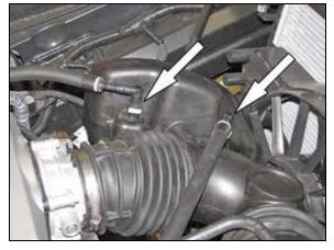
3. Release the grey locking tabs securing the crank case vent and oil tank vent tubes to the factory intake hoses and then disconnect the crank case hoses from the intake tube.
