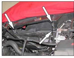
14. Install the three provided rubber mounted studs onto the heat shield mounting location as shown.
