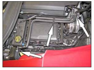
4. On vehicles that are equipped with a "Dry Sump" oiling system, release the grey locking tap securing the oil tank vent hose to the oil tank, then unhook the oil tank vent hose from the two retaining clips and remove the hose from the vehicle.
