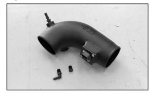
24. Install the provided vent fittings into the into the  $K\&N^{\otimes}$  intake tube as shown.
