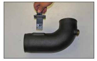
23. Install the mass air sensor assembly into the K&N<sup>®</sup> intake tube and secure with provided hardware.
