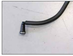
30. Cut the provided crank case vent hose to a length of 15" and install onto the factory 90° quick disconnect fitting.
