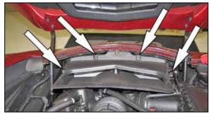
2. Remove the four bolts that secure the air extraction duct to the radiator and then remove the duct from the vehicle.
