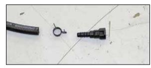
10. Assemble the provided coolant hose (08636), quick disconnect fitting and clamps. Install one clamp 1.5" from the open end of the provided coolant hose.
