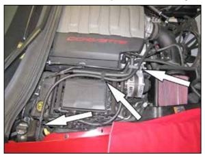
28. On vehicles that are equipped with a "Dry Sump" oiling system, install the crank case vent hose assembly onto the oil tank and then route it through the factory retaining clips and then connect the open end to the 90° fitting installed into the K&N® intake tube.
