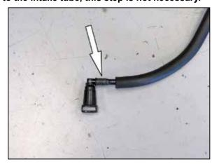
29. On vehicles equipped with a "Wet Sump" oiling system, separate the nylon crank case vent hose from the 90° quick disconnect fitting.
