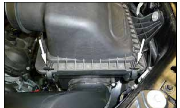
6. Release the two locking clips that secure the upper air filter housing and then remove the upper housing from the vehicle.
