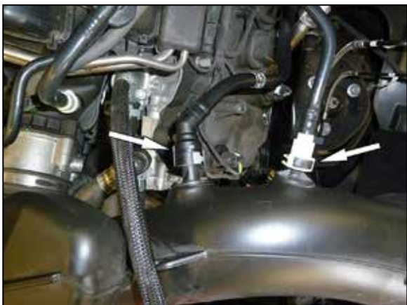
2. Disconnect the EVAP and CCV hoses from the factory intake tube.
