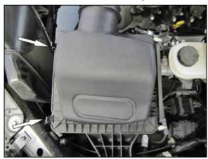
4. Release the two clips that secure the upper air filter housing and then remove the upper housing and factory air filter.
