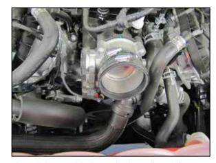
7. Install the provided coupler hose (08615) onto the throttle body and secure with the provided hose clamp.
