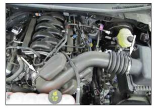
3. Loosen the hose clamps that secure the factory intake tube to the air filter housing and throttle body and then remove the intake tube from the vehicle.
