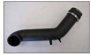
6. Install the Provided vent fittings into the K&N intake tube as shown. Install the provided hump coupler (08683) onto the intake tube and secure with the provided hose clamp.
