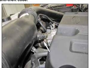
2. Disconnect the inlet air temperature sensor.
