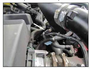
10. Reconnect the inlet air temperature sensor electrical connection.
