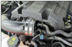
7. Install the provided coupler hoses onto the turbo inlet tubes and secure with the provided hose clamps.
