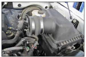
6. Install the provided hump hose (08683) onto the air filter housing and secure with the provided hose clamp.
