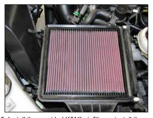
5. Install the provided K&N® air filter, reinstall the upper air filter housing and secure with the factory clips.
