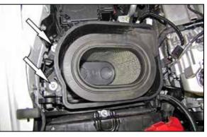
4. Remove the two bolts that secure the lower air filter housing to the mounting bracket and remove the lower filter housing.
