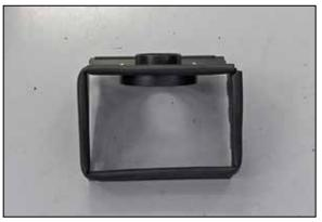
9. Install the K&N® filter adapter into the heat shield and secure with the provided hardware.
