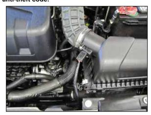
2. Release the red locking tab and then disconnect inlet air temperature sensor electrical connection.
