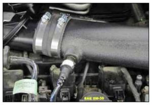
20. Connect the EVAP vent line to the quick disconnect fitting installed into the K&N® intake tube.
