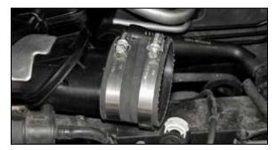
14. Install the coupling hose (08690) onto the turbo inlet and secure with the provided hardware.
