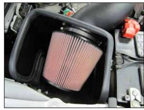
20. Install the K&N® air filter onto the intake tube and secure with the provided hose clamp.
