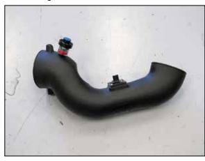
18. Install the filter minder using the provided grommet into the  $K\&N^{\otimes}$  intake tube.
