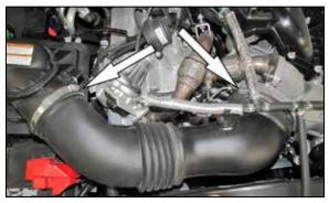
3. Loosen the hose clamps that secure the factory intake tube to the turbo inlet and air filter housing. Then remove the intake tube from the vehicle.
