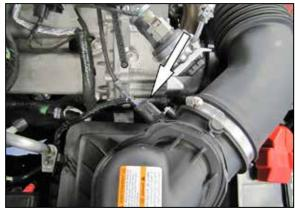
2. Release the locking tab and then disconnect the mass air sensor electrical connection.
