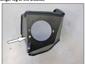
10. Attach the bracket assembly onto the heat shield as shown and secure with the provided hardware.
