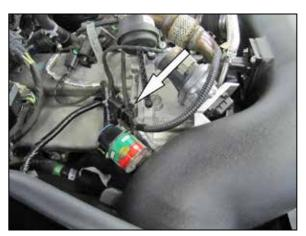
21. Connect the provided mass air sensor extension harness to the factory wiring harness and then into mass air sensor. Using the provided tie wrap, secure the extension harness to the factory harness so that it does not interfere with and potentially moving parts as shown.
