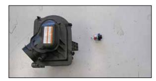
17. Remove the factory filter minder from the air filter housing.
