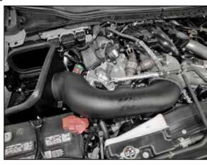
19. Install the intake tube into the heat shield and then into the coupling hose at the turbo inlet, adjust the tube for best fit and then install the provided bolts through the heat shield to secure the tube to the heat shield. Then secure the tube to the coupling hose with the provided hose clamp.
