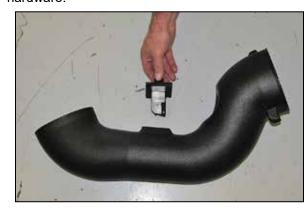
16. Install the mass air sensor assembly into the K&N® intake tube as shown and secure with the provided hardware.
