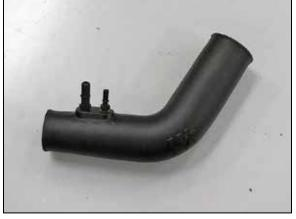
13. Install Quick disconnect fittings into the K&N<sup>®</sup> intake tube as shown.
