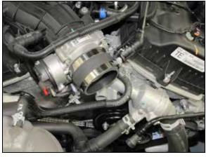
12. Install the provided straight coupler (08711) onto the throttle body and secure with the provided hose clamp.
