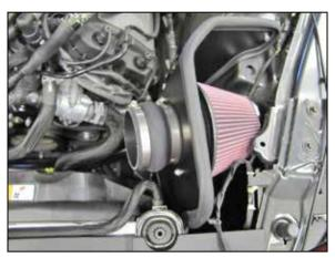
11. Install the provided hump coupler (08699) onto the filter adapter and secure with the provided hose clamp.
