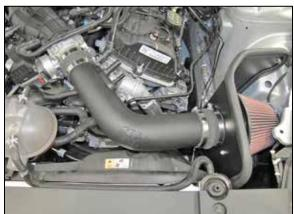
14. Install the intake tube fully into the hump
