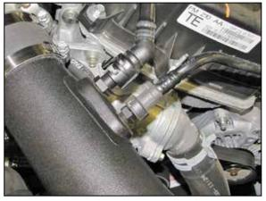
15. Connect the crank case vent and EVAP vent lines to the fittings installed into the K&N<sup>®</sup> intake tube.
