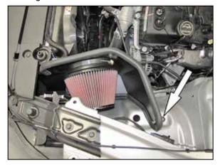
10. Flex the heat shield back and install the K&N<sup>®</sup> air filter onto the adapter then secure the filter
