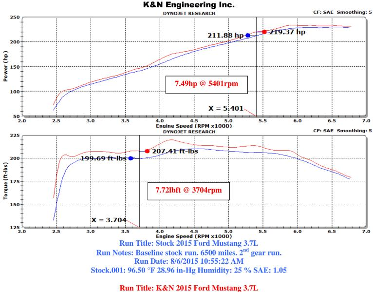
Run Notes: K&N intake kit #63-2594 installed. 6500 miles. 2<sup>nd</sup> gear run. Run Date: 8/6/2015 12:59:51 PM K&N.002: 106.74 °F 29.00 in-Hg Humidity: 17 % SAE: 1.06
