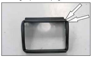
9. Install the large edge trim onto the top of the heat shield as shown.
