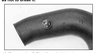
18. Remove the O-Ring from the inlet air temperature sensor, then install it into the grommet installed into the K&N® intake tube.
