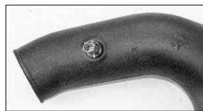
18. Remove the O-Ring from the inlet air temperature sensor and then install it into the grommet installed into the  $K\&N^{\otimes}$  intake tube.
