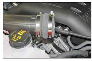
15. Install the provided coupling hose (087121) onto the passenger side turbo inlet tube and secure with the provided hose clamp.
