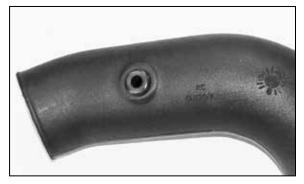
16. Install the provided grommet into the  $K\&N^{\otimes}$  intake tube as shown.
