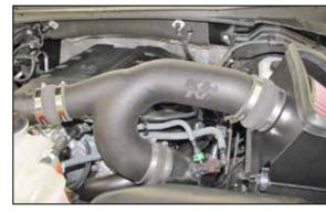
19. Install the K&N® intake tube into the turbo inlet hoses and then into the hose at the throttle body, adjust the tube for best fit and then secure with the provided hose clamps.
