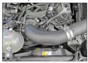
16. Install the K&N® intake tube along with the coupling hose (08536) into the hump hose at the throttle body and then onto the upper air box housing. Secure the hoses with the provided hose clamps.
