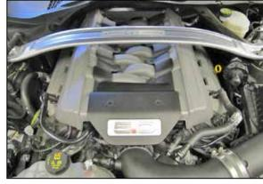
19. Reinstall the Engine cover onto its mounting studs.
