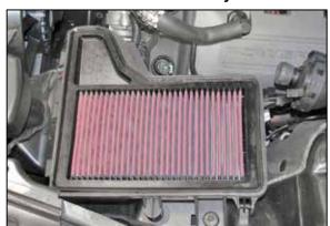
10. Install the  $K\&N^{\otimes}$  air filter into the lower air filter housing.
