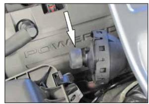
6. Install the provided cap onto the sound drum as shown.
