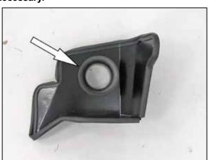
10. Install the filter adapter into the heat shield as shown.
