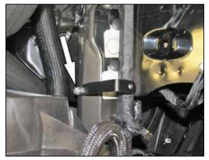
12. Install the heat shield mounting bracket onto the inner frame rail using the provided hardware. NOTE: Use the existing threaded hole in the frame rail.
