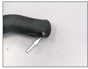
18. Remove the O-Ring from the factory temperature sensor and then install the sensor into the grommet installed into the K&N® intake tube.
