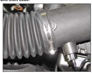
2. Loosen the hose clamp securing the factory intake tube to the air filter housing.
