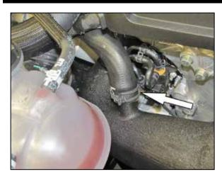
22. Install the BOV hose onto the K&N<sup>®</sup> intake tube and release the factory spring clip.
