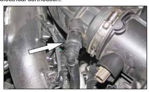
3. Disconnect the crank case vent connection.
