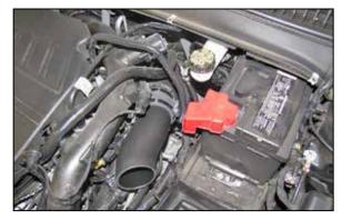
13. Install the K&N $^{\odot}$  intake tube into the coupling hose at the turbo but do not tighten at this time.
