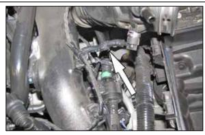
6. Disconnect the solenoid vent hose from the fitting installed into the factory intake tube.
