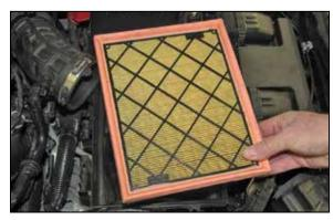
5. Release the two upper air box retaining clips and then remove the upper air box and stock air filter.
