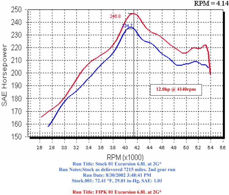
Run Notes: K&N Intake Kit installed. 7215 miles. 2nd gear run. Run Date: 8/30/2002 3:48:41 PM FIPK.002: 72.92 °F, 29.01 in-Hg, SAE: 1.01
