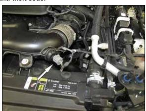
2. Disconnect the inlet air temperature sensor electrical connection and unhook the wiring harness from the intake tube.
