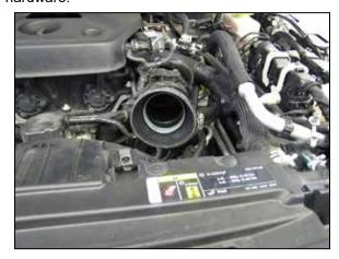
16. Install the provided step coupler onto the throttle body and secure with the provided hose clamp.
