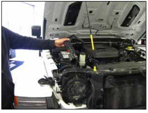
8. Remove the two bolts that secure the fresh air duct to the core support and then remove the duct from the vehicle.
