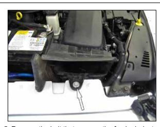
5. Remove the bolt that secures the fresh air duct to the fender. Remove the complete intake system from the vehicle.
