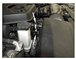
3. Depress the locking tab and disconnect the two vent lines from the air filter housing.
