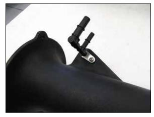
12. Install the O-ring onto the ejector fitting provided and then install the fitting into the K&N® intake tube. Secure the fitting with the clip and hardware provided.
