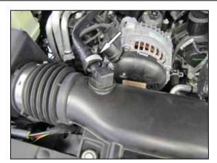
3. Disconnect the crank case vent line.
