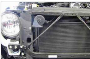
9. Reinstall core support brace onto the core support.
