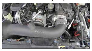
18. Reconnect the crank case vent line onto the quick connect fitting and reconnect the inlet temp sensor electrical connector onto the temp sensor.
