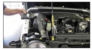
8. Remove the two bolts that secure the inlet scoop to the core support and remove inlet scoop.
