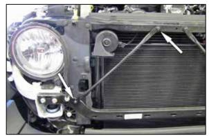
7. Remove the two bolts that secure the core support brace to the core support and remove brace.
