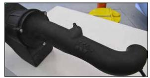
15. Install the K&N $^{\circ}$  intake tube assembly onto the K&N $^{\circ}$  airbox with provided hardware. Note the orientation of the K&N $^{\circ}$  intake tube.
