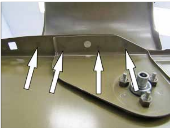
49. Use a center punch to mark the four spot welds which hold the cowl corner cap to the fender. Then drill out the spot welds to remove the cowl cap from the fender. NOTE: Start with a 1/8" drill and work up to an 11/32" bit until the spot weld is removed. This will help to prevent any unnecessary damage to the fender.
