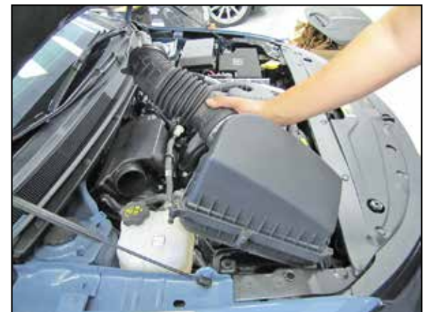
5. Separate the factory intake tube from the intake plenum and then lift up the complete upper air filter housing to dislodge it from the mounting grommets and remove it from the vehicle. NOTE: K&N Engineering, Inc., recommends that customers do not discard factory air intake.
