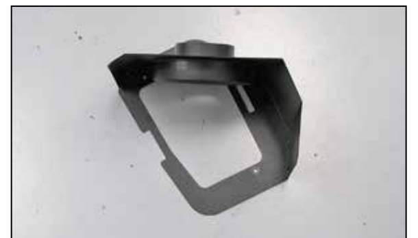
6. Install the provided air filter adapter into the heat shield and secure with the provided hardware.
