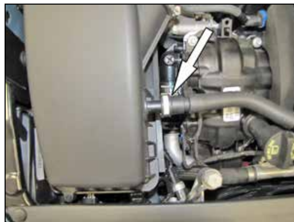
4. Depress the locking tab and then disconnect the crank case vent hose assembly from the air filter housing.
