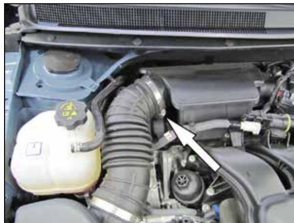
3. Loosen the hose clamp that secures the factory intake tube to the intake plenum.
