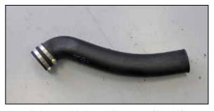
7. Install the provided coupling hose (08690) halfway onto the K&N $^{\otimes}$  intake tube and secure with the provided hose clamp as shown.
