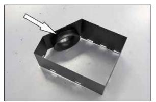
12. Install the provided radius adapter into the heat shield and secure with the provided hardware.
