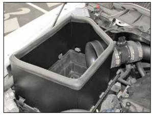
14. Install the heat shield onto the lower air filter housing and secure with the factory retaining clips. NOTE: It is best to install the coupling hose onto the filter adapter as the heat shield is being set into position.
