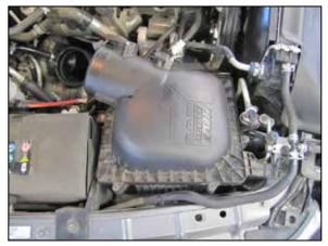
9. Reinstall air box lid onto air box base.
