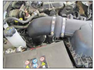
11. Install K&N<sup>®</sup> intake tube into the factory turbo inlet hose and then into coupling hose (08695). Secure K&N<sup>®</sup> intake tube with provided hose clamps.
