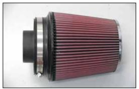
24. Install the filter adapter into the air filter as shown and secure with the provided hose clamp. NOTE: Drycharger<sup>®</sup> air filter wrap; part # RF-1014DK is available to purchase separately.
