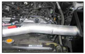
22. Install the K&N<sup>®</sup> intake tube into the silicone hose at the throttle body and align with the tube mounting bracket installed in step #16. Secure with the provided hardware and hose clamp.
