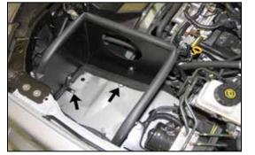
Install the heat shield assembly into the vehicle and secure with the provided hardware.
