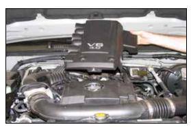
4. Lift firmly on the engine cover to dislodge it from the mounting grommets, and then remove the cover from the engine as shown.
