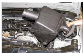
10. Pull firmly on the airbox to dislodge it from the mounting grommets and remove it from the vehicle. NOTE: K&N Engineering, Inc., recommends that customers do not discard factory air intake.
