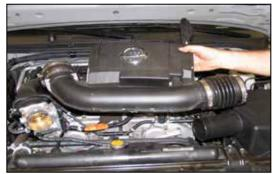
2. Disconnect the mass air sensor electrical connection and unhook the harness from the airbox.
