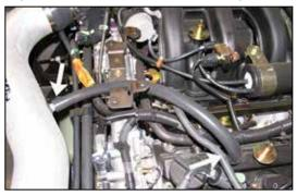
23. Attach the provided silicone crankcase vent hose to the valve cover and  $K\&N^{\ensuremath{\mathbb{R}}}$  intake tube as shown.
