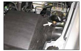
9. Remove the airbox retaining bolt shown.
