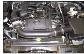
7. Loosen the two hose clamps shown which secure the stock intake tube to the airbox and to the throttle body.
