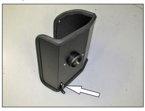
12. Install the provided heat shield mounting bracket (07805) onto the heat shield as shown using the provided hardware.
