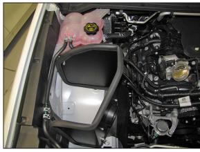
15. Install the heat shield so that the brackets set onto the coolant reservoir stud and the air filter housing mounting stud then secure the heat shield with the factory mounting nuts removed earlier.
