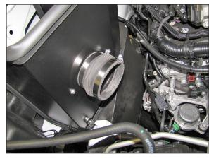
16. Install the provided hump coupler (06899) onto the filter adapter and secure with the provided hose clamp.
