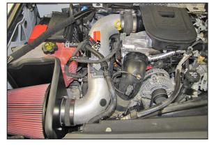
17. Install the K&N® intake tube into the hump hose at the turbo inlet and then into the hose at the filter adapter, adjust the tube for best fit and then secure with the provided hose clamp.
