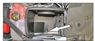
10. Install the heat shield assembly into the vehicle and secure with one of the factory bolts removed in step #7 to the fender.
