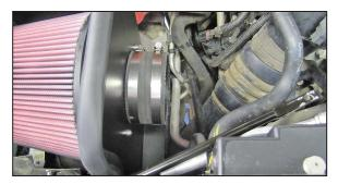
12. Install the coupling hose (08761) onto the filter adapter and secure with the provided hose clamp.
