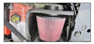
11. Flex the heat shield back and then install the K&N® air filter onto the filter adapter and secure with the provided hose clamp. Secure the heat shield with two of the factory bolts removed in step #7.
