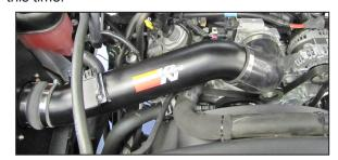
17. Install the K&N® intake tube into the coupling hoses and then adjust the tube for best fit. Secure the hoses and tube with the provided hose clamps.
