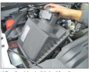
6. Lift up the air box to dislodge it from the mounting grommets, and then remove it from the vehicle as shown.
