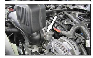
5. Loosen the hose clamps that secure the intake tube to the throttle body and air filter housing. Unhook the radiator hose clip from the intake tube and then remove the intake tube from the vehicle.
