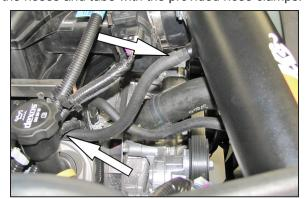
18. Install the provided crank case vent hose onto the fitting installed into the K&N® intake tube and then onto the valve cover port. Secure the hose to the valve cover port with the provided hose clamp.
