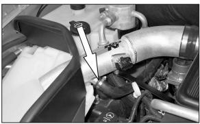
17. Cut the air injection hose at the location marked in step #16. Then install the hose onto the K&N<sup>®</sup> intake tube and secure with the provided hose clamp
