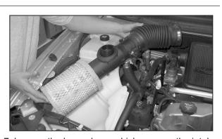
7. Loosen the hose clamp which secures the intake tube to the intake plenum and then remove the complete intake system as shown.
