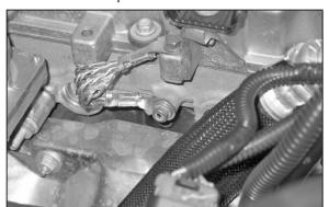
11. Remove the engine ground strap bolt shown. **NOTE: This bolt will be reused.**
