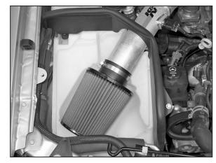
18. Install the K&N® air filter onto the K&N® intake tube and secure with the provided hose clamp.
