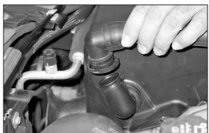
3. Depress the locking tabs and disconnect the air injection hose from the upper air box housing as shown.
