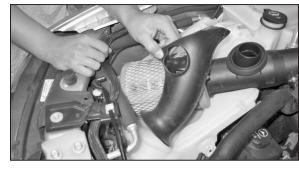
6. Remove the fresh air supply duct from the lower air box housing as shown.
