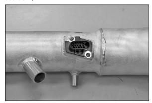
14. Install the mass air sensor into the K&N® intake tube and secure with the provided hardware.
