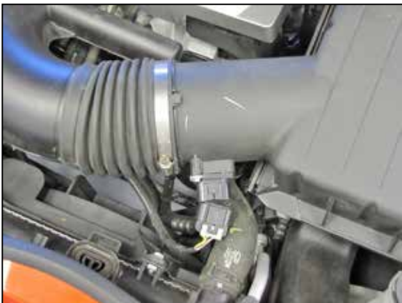
2. Disconnect the mass air sensor electrical connection.
