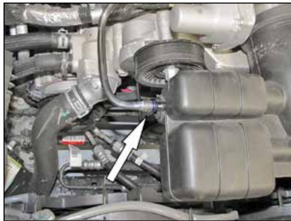
4. Disconnect the crank case vent tube from the intake resonator as shown.
