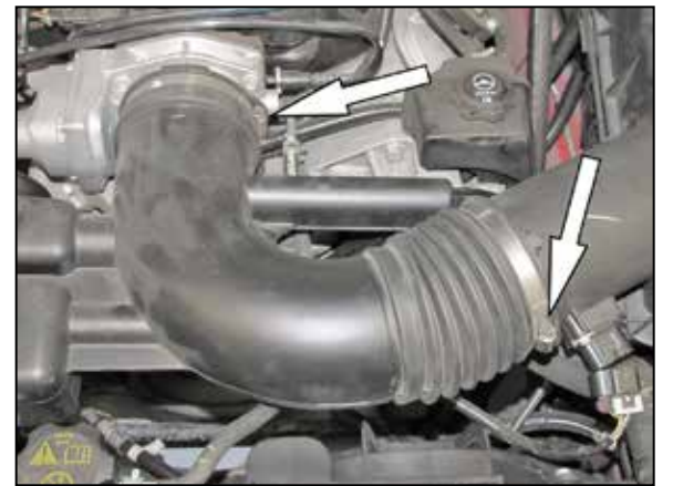
5. Loosen the hose clamps which secure the stock intake tube to the air box and throttle body.
