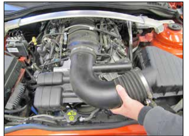
6. Remove the stock intake tube as shown.
